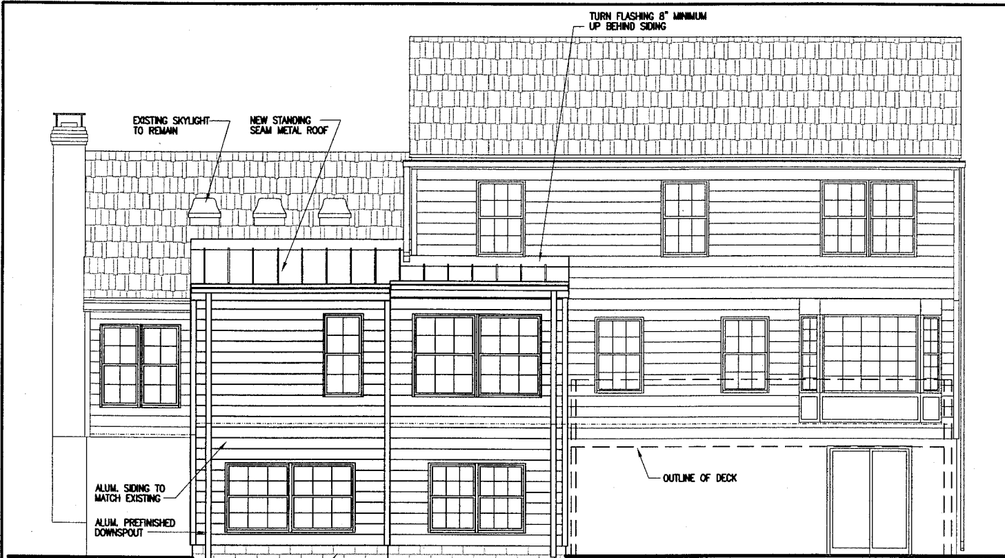
1 REAR ELEVATION A-3 SCALE: 1/4" = 1'-0" EXISTING BUILDING ADDITION CONCRETE BLOCK FOUNDATION WALL PARGED AND PAINTED ADDITION EXISTING BUILDING
